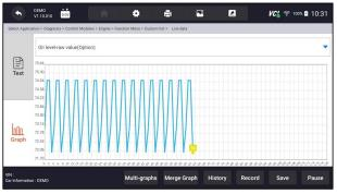
Figure 9-20 Sample PID Graph Screen
