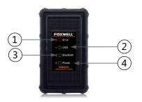
Figure 2-5 Front View of VCI dongle
