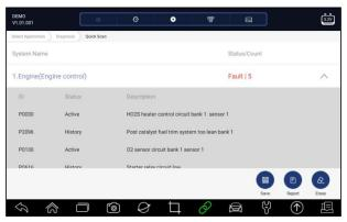
Figure 5-4 Sample Quick Scan Complete Screen
