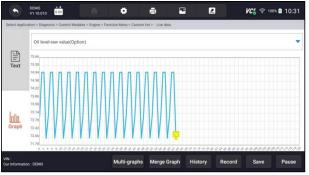
Figure 5-20 Sample PID Graph Screen
