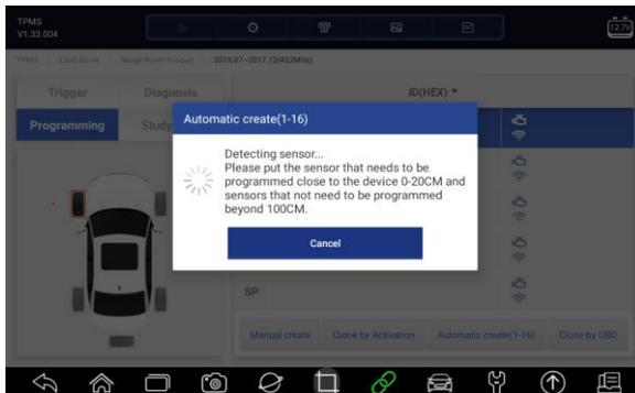
Figure 7- 13 Sample Automatic Create Function Screen
