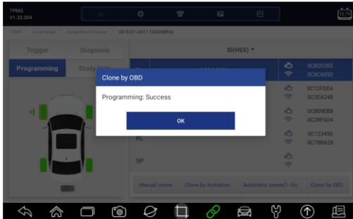
Figure 7- 16 Sample Copy by OBD Function Screen
