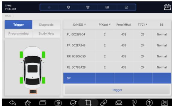
Figure 7- 5 Sample Trigger TPMS Screen
