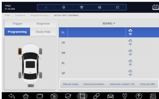
Figure 7- 7 Sample Programming Function Screen
