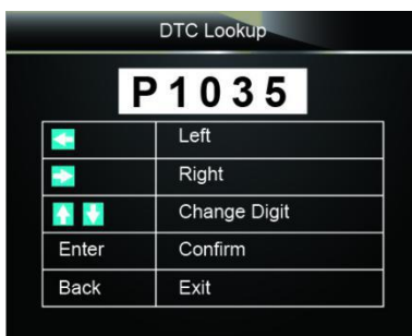
Figure 6-2 Sample DTC Lookup Screen
